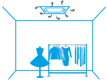
Air distribution with a dusty filter
